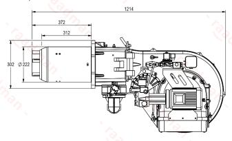
Suggested boiler flange diameter = 235 mm
