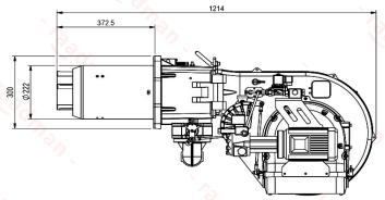
Suggested boiler flange diameter = 235 mm
