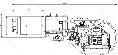
Suggested boiler flange diameter = 331 mm
