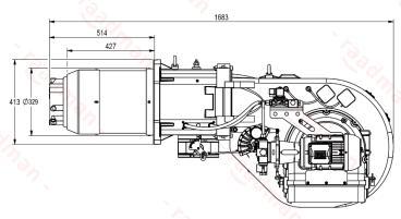
Suggested boiler flange diameter = 331 mm
