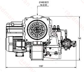
Suggested boiler flange diameter = 340 mm
