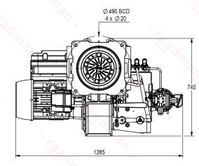
Suggested boiler flange diameter = 340 mm
